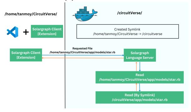
To work on this, we need to provide the host current directory path to the container, we are going to do this by setting an environment variable in docker-compose.yml file for web service.
